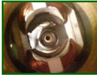
A motor with the rotor coils removed exposing the stator coils
